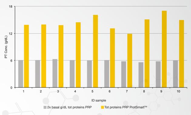
Total protein concentration in basal PRP and concentrated PRP measured by ProtSmart<sup>™</sup>. The total plasma proteins including autologous growth factors increase their concentration by about 2.2-3 times compared to the basal PRP concentration obtained by a single centrifugation.
